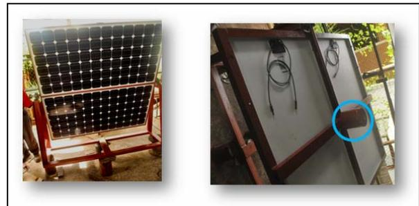
Fig. 5: The solar panel affixed to the frame (left). The counter-weight (circled, right).
