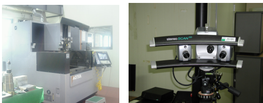
Fig. 16: Manufacturing machine to process gears (W-EDM, AQ750L) and Photography of Reverse Engineering System (StereoSCAN 3D )
