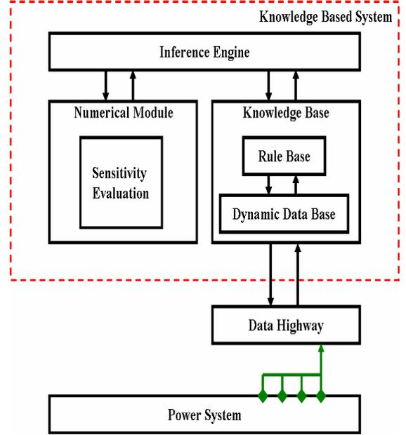
Figure 3: The structure of the intelligent voltage control system
