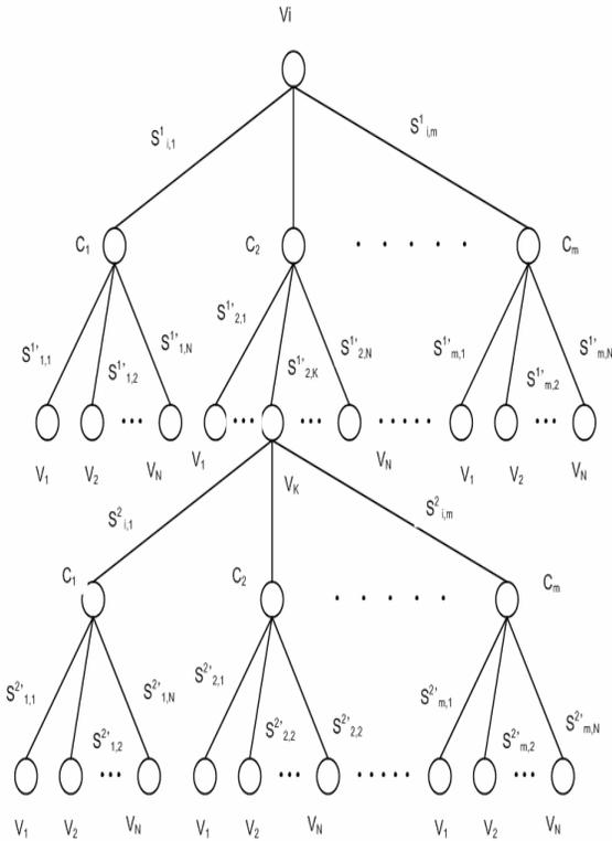
Figure 2: The voltage control state-space model
