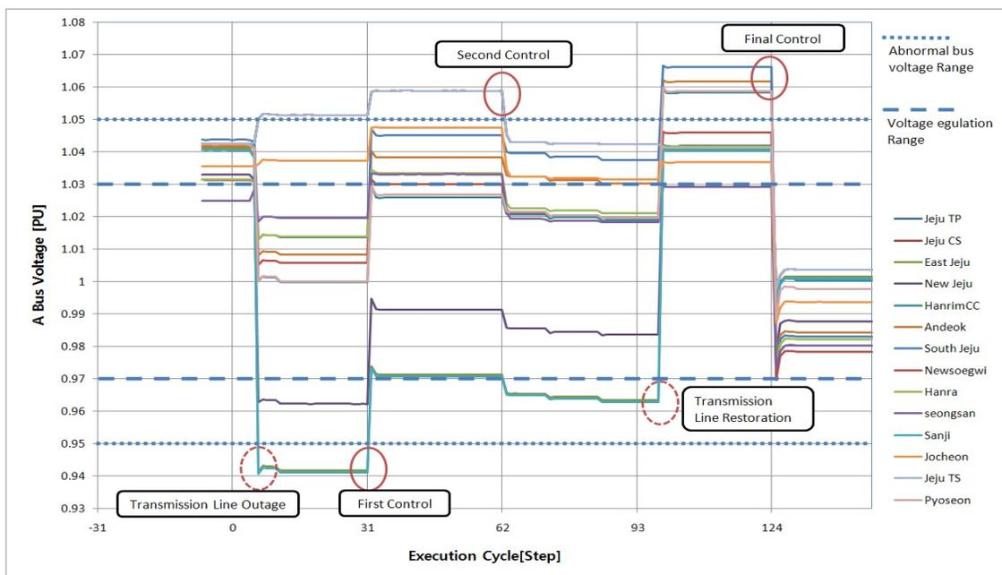
Figure 6: The 154kV bus voltage profile in the Jeju power system
