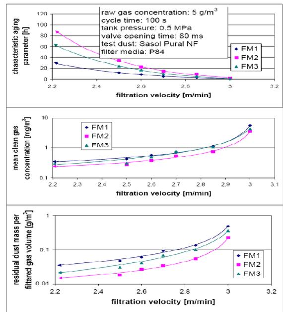
Figure 16. Characteristic aging parameter, mean clean gas concentration and residual dust mass per filtering gas volume for different filtration velocities
