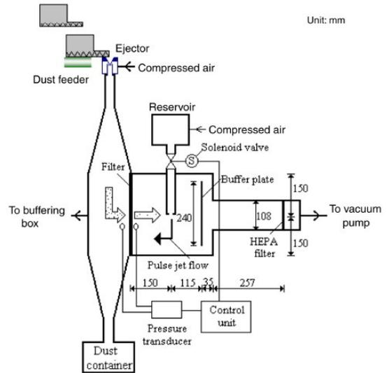
Figure 4. Japanese test standard JIS Z8909-1 [5]
