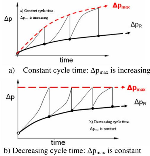
Figure 12. Pressure drop development over time
