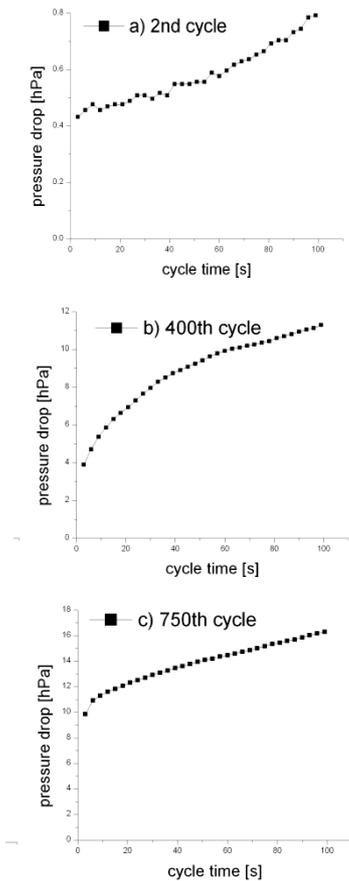
Figure 11. Pressure drop increase versus cycle time for an aging test with 2.5 m/min filtration velocity and 100 s cycle time
