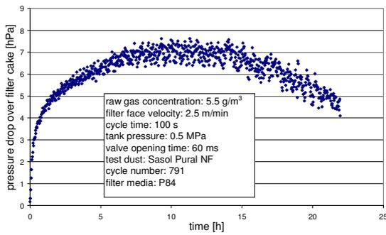
Figure 10. Cake pressure drop over the test time
