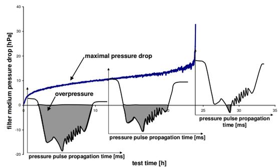
Figure 13. Pressure drop during cleaning by back pulse at different test times
