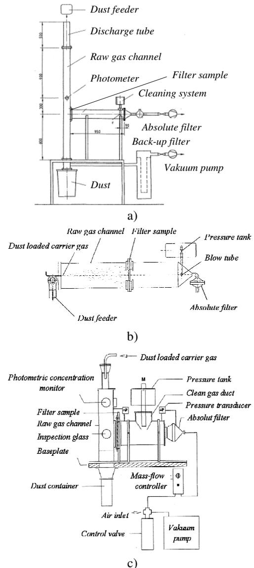
Figure 5. German test standard VDI 3926 [6]
