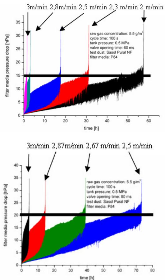
Figure 9. Aging test with different filtration velocities and two valve opening times
