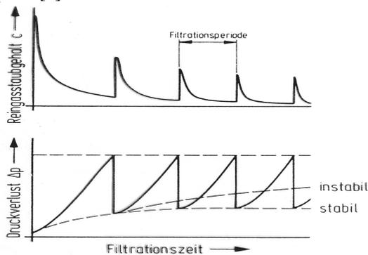
Figure 3. Pressure drop and concentration over time for a bag house filter [3]
