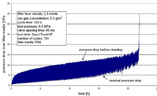
Figure 7. Pressure drop over time for an aging test (100s cycle time, 2.5 m/min filtration velocity)
