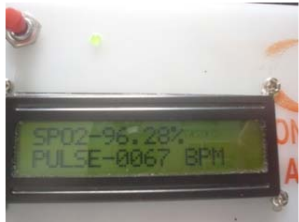
Figure 8: LCD display showing SpO 2 and Pulse Rate
