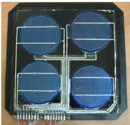
Fig. 16: PV/T receiving element of hybrid collector module
