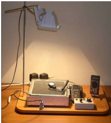
Fig. 15: Lab set for study of solar thermal collector
