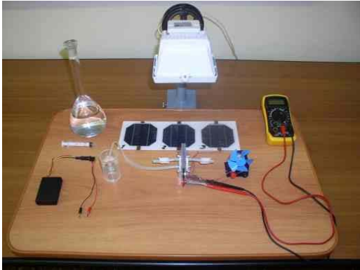
Fig. 14: Lab equipment for study of solar-hydrogen system with reversible fuel cell
