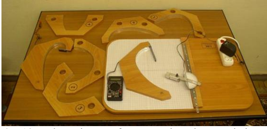
Fig. 13: Lab equipment for measuring characteristics of concentrators
