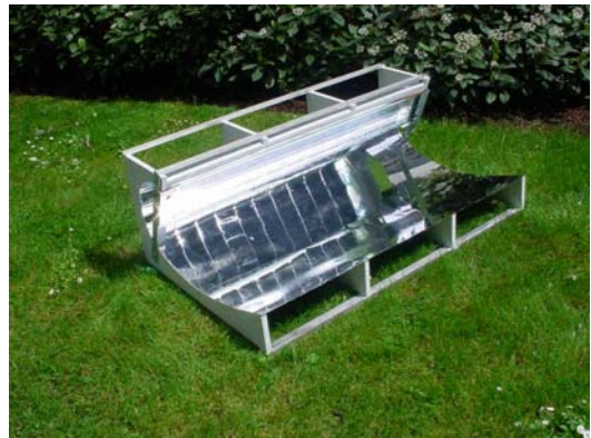
Fig. 8: The photo of the concentrator with bifacial receiver in horizontal working position
