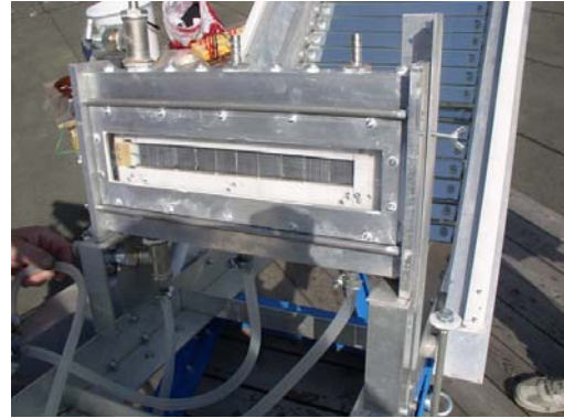
Fig. 11: Experimental PVT receiver in concentrator
