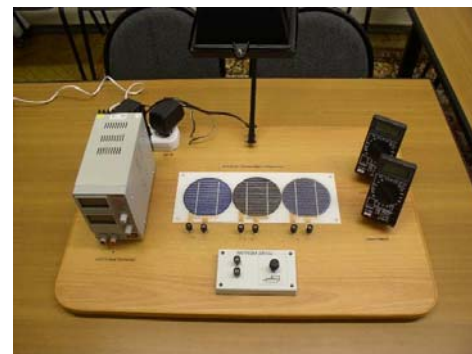
Fig. 12: Lab equipment for measuring characteristics of solar cells
