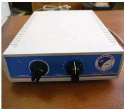
Fig. 21: Portable receiver of satellite space images of the Earth
