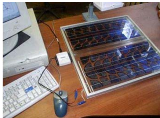
Fig. 19: Solar PV module developed for schools with test equipment
