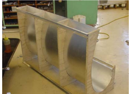
Fig. 7: Photo of concentrator from Al/plywood frame
