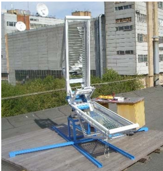
Fig. 10: Experimental concentrator for VEI PVT system
