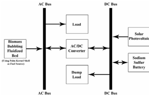
Figure 1. Integrated Electricity System Configuration
