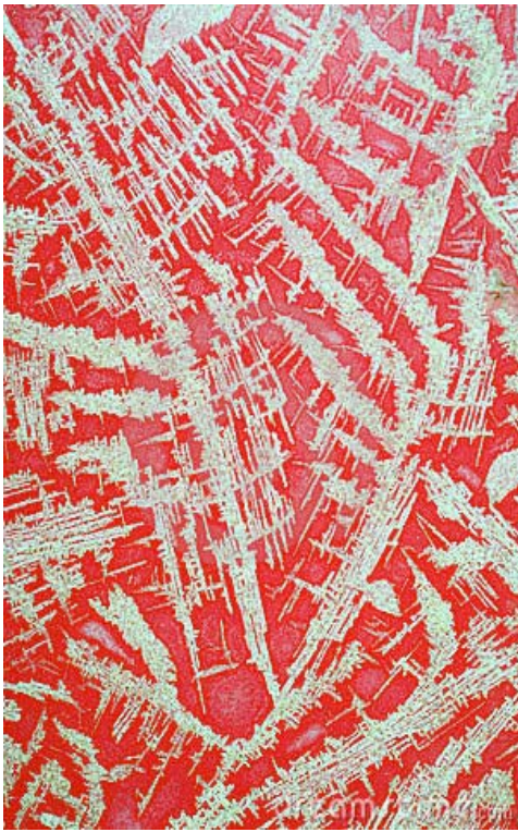
Photo 3. Dried material after ethyl acetate extraction of Punctelia thalli . The material formed flat red crystals on the surface of the dish.
