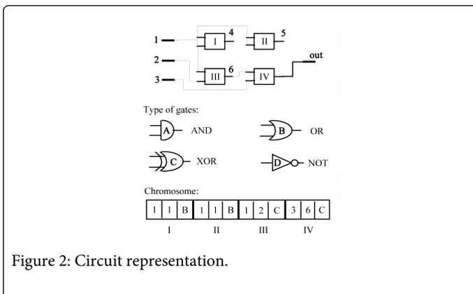
The first interesting aspect of this problem is the encoding of solutions as strings of bits, each string being a chromosome that the GA can evolve. Figure 2 explains the main idea used for this purpose. Each chromosome contains the whole information about the connections between inputs and outputs of the gates. Each gate contain three fields: the two first fields refer to each of the inputs used, and the third is the type of the gate [11].
