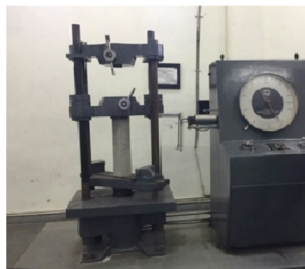
Figure 2: Testing of Rectangular column on UTM.
