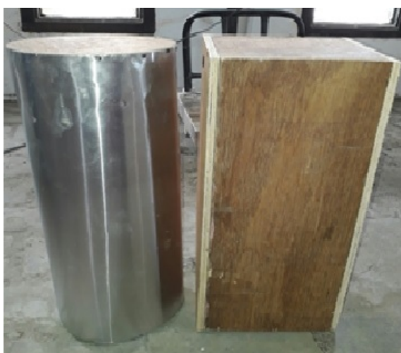
Figure 1: Circular mould=15 cm × 40 cm, Rectangular mould=15 cm × 15 cm × 40 cm.
